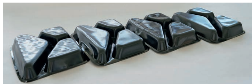
Fig. 6. Oven tests at 200°C for 20 min: rCPET trays (from left to right: rolls 2, 3, 4, 5); upper heater at 250°C; upper and lower heating, lower heater at 270°C (© Illig)
